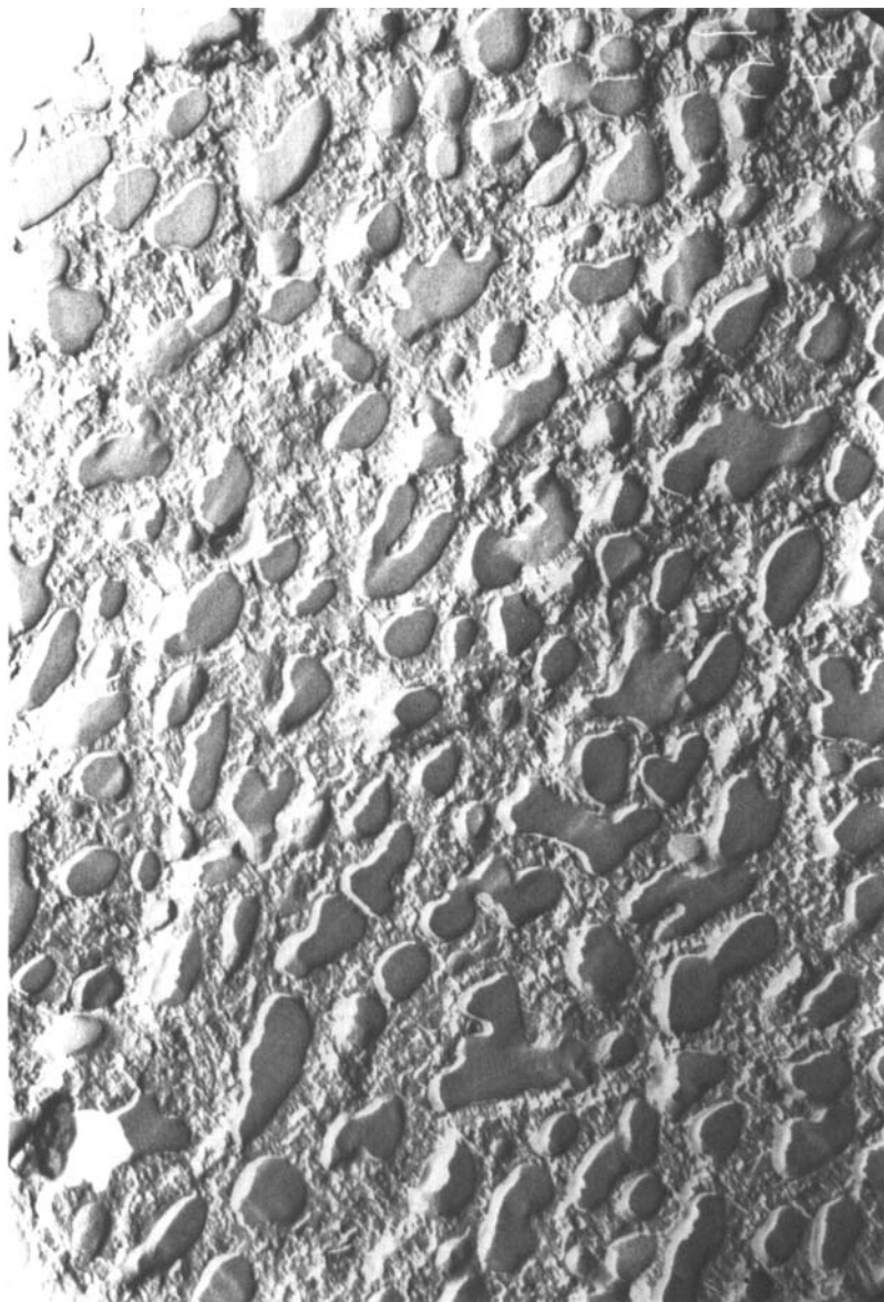
FIGURE 3 Electron micrograph of replica obtained from N_L phase with etching (magnification, \times 20,000 ).
