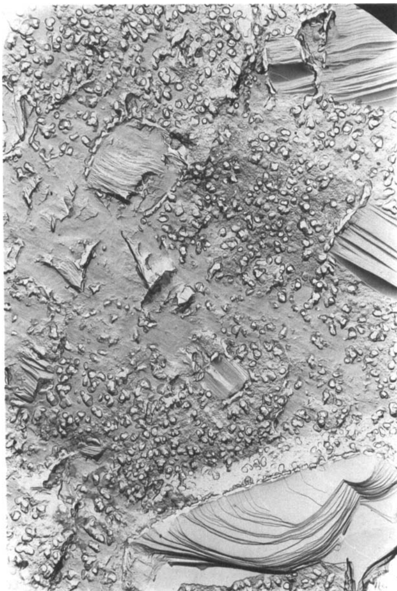
FIGURE 5 Electron micrograph of replica obtained from CG phase with etching (magnification, \times 8,000 ).
